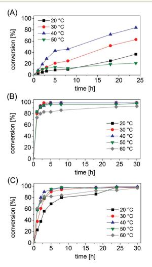
Fig. 1 Progress of the reaction vs. the time for the reductive amination of: (A) 1a using Bb-PhAmDH (46  $\mu$ M), (B) 24a using by Rs-PhAmDH (48  $\mu$ M), and (C) 10a using Ch1-AmDH (33  $\mu$ M). The study was carried out at different temperatures: 20 °C (black), 30 °C (red), and 40 °C (blue), 50 °C (green), and 60 °C (grey). Reaction conditions: 0.5 mL, 50 mM substrate, ammonium formate buffer (1.00 M, pH 8.5), FDH (14  $\mu$ M).
