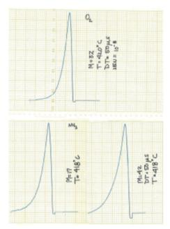
Fig. 2 Original TAP pulse responses for O2, NH3 and C3H6 over SiO2 obtained with a chart recorder. 30 The pulses are plotted from right to left and the scale is 1 cm equal to 0.5 s.
