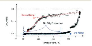
Fig. 11 CO<sub>2</sub> production observed from atmospheric flow experiment over a single Pt particle. The CO2 produced while increasing reactor temperature is less than the CO<sub>2</sub> produced during reactor temperature decrease as shown by the counter-clockwise hysteresis loop. 18
