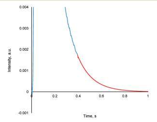
Fig. 13 A truncated argon pulse response (blue) which has had its remainder generated through tail expansion (red).
