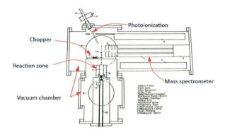
Fig. 1 Schematic of TAP system which appeared in original research proposal in 1977 by J. T. Gleaves.<sup>27</sup>
