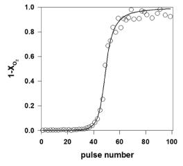
Fig. 6 Oxygen breakthrough curve, i.e. fraction of oxygen released from TAP reactor after each subsequent pulse over a Pd/SiO<sub>2</sub> catalyst (a series of  $2 \times 10^{15}$  O<sub>2</sub> molecules per pulse are introduced over 10 mg of 1.0 wt% Pd/SiO<sub>2</sub> catalyst at T = 100 °C). Open circles: experimental data, line: model.31
