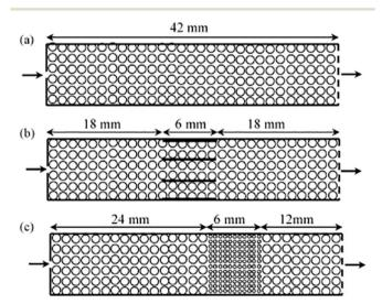
Fig. 8 Schematics of one-zone inert (a), three-zone monolith (b), and three-zone powder (c) configurations. 127
