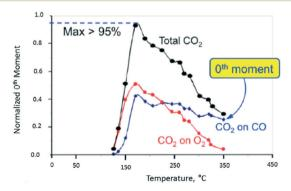
Fig. 10 CO<sub>2</sub> production observed from vacuum pump-probe experiment over a single Pt particle. The black line represents the total  $CO_2$  yield. The red and blue lines represent the  $CO_2$  yield on the oxygen pulse and CO pulse, respectively.18
