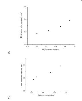
Fig. 9 Galactose isomerization first order rate constant vs. a) molar Mg content and b) basicity of magnesium aluminates. Reaction conditions: 110 °C,  $m_{cat}$  = 9.2 g, 5 bar, 1000 rpm and calcination temperature = 680 °C.
