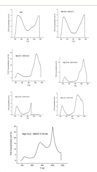
Fig. 3 CO<sub>2</sub> TPD for the catalysts in Table 3.
