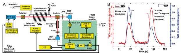
(A) Schematic configuration of a FRS system. (B) Measurement of <sup>15</sup>NO (red) and <sup>14</sup>NO (blue) concentration after chemical conversion of nitrite/ nitrate from patient's urine samples obtained before and after <sup>15</sup>N labeled arginine was introduced. Reproduced from ref. 132 with permission from Nature Publishing Group, copyright 2015.
