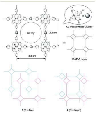
Scheme 1 Construction of P-MOFs incorporating cavities.
