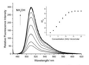
Fig. 1 Fluorescence changes observed for probe 1 (0.5  $\mu$ M) during the addition of HA (0–20  $\mu$ M), in 1% DMSO PBS Buffer at pH 7.4.  $\lambda_{ex}$  = 465 nm, with a 5 min delay between additions of HA. Inset: Relative fluorescence changes (I/I<sub>0</sub>) as a function of HA concentration (0-20  $\mu$ M)
