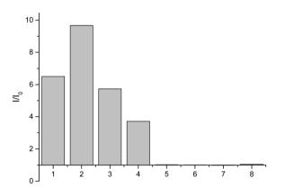
Fig. 2 Selectivity of probe  $\mathbf{1}$  (0.5  $\mu$ M) towards various hydroxylamines (1) hydroxylamine, (2) N-(methyl)hydroxylamine, (3) N-(benzyl)hydroxylamine, (4) N-(propargyl)hydroxylamine, (5) N-(tert-butyl)hydroxylamine, (6) O-(benzyl)hydroxylamine, (7) N-(phenyl)hydroxylamine, (8) blank. 15 min incubation with each analyte (50  $\mu$ M) in PBS buffer, 1% DMSO pH = 7.4. Slit width ex = 5 nm, em = 2.5 nm.  $\lambda_{ex}$  = 465 nm,  $\lambda_{em}$  = 510 nm.
