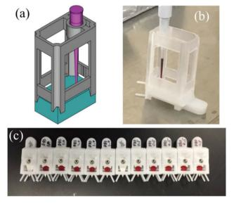
Fig. 3 A spotting apparatus was designed (a) and used to spot 12 µL of blood onto the Prosolia paper spray cartridges (b, c).
