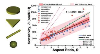
Fig. 6 Bulk sensitivity (in units of nm RIU<sup>-1</sup>) of different types of plasmonic nanostructures supporting LSP resonances with different aspect ratios. Different symbols correspond to different structures. Reproduced with permission from A. U. Khan *et al.*, *J. Phys. Chem. C*, 2016, **120**, 19353–19364 (ref. 59). Copyright 2016 American Chemical Society. For the meaning of the different colours, lines and shades the reader is referred to ref. 59.
