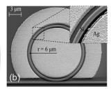
Fig. 10 Hybrid WGM structures for bulk refractive index sensing. (a) SOI ring resonator decorated with metallic nanodisks along the circumference. Reproduced from ref. 89 with permission from The Royal Society of Chemistry. (b) Metal-dielectric double slot SOI ring resonator. The inset shows the gap between the silicon ring and the surrounding silver plate, which is the region of accumulation of the electromagnetic field. Reproduced from ref. 94.
