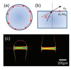
Fig. 1 (a) Sketch of a light ray travelling inside a spherical dielectric cavity. (b) Illustration of the Snell law: the refractive index of the cavity material is denoted with  $n_1$ , that of the surrounding medium with  $n_2$ , and the critical angle for total internal reflection with  $\theta_c$ . (c) Optical picture of the standing wave profile in a resonant double sphere cavity system fed by a tapered optical fibre. Reproduced from ref. 11.
