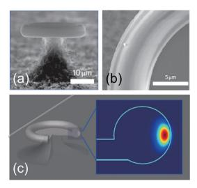
Fig. 11 Single particle detection with a purely photonic WGM resonator. (a) SEM image of a micro-toroid (diameter: 40  $\mu$ m) used for the optical measurement. (b) SEM detail of a PS nanoparticle (diameter: 300 nm) bound to the surface of the toroid. (c) 3D rendering of the micro-toroid employed in the numerical simulations and cross section of the electric field of the WGM mode. Reproduced and adapted from ref. 28.
