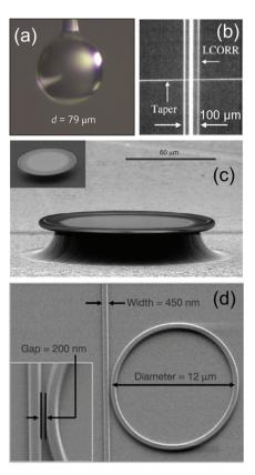
Fig. 4 (a) Optical picture of a glass microsphere resonator attached to an optical fibre. Reproduced from ref. 25. (b) Picture of a capillary resonator. Adapted from ref. 35. (c) SEM image of a fused silica toroidal cavity on a silica substrate. Reproduced from ref. 36. (d) SEM image of a silicon ring resonator on a silicon-on-insulator wafer. Reproduced from ref. 37.
