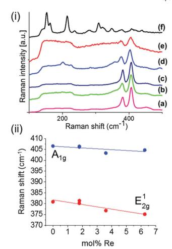
Fig. 7 (i) Raman spectra of  $Mo_{1-x}Re_xS_2$  ( $0 \le x \le 0.06$ ) thin films deposited at 475 °C by AA-CVD. (a) MoS2, (b) 1.79 mol% Re, (c) 1.80 mol% Re, (d) 3.60 mol% Re, (e) 6.25 mol% Re, (f) ReS2. Spectra are stacked for clarity. (ii) Dependence of the Raman shift of the  $E_{2g}^1$  and  $A_{1g}$  optical modes of  $Mo_{1-x}Re_xS_2$  on the amount of Re-dopant.
