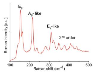
Fig. 3 The Raman spectrum of as-deposited ReS<sub>2</sub> thin films produced by AA-CVD at 475 °C. The profile is consistent with the Raman spectrum of ReS<sub>2</sub> previously reported.<sup>28,29</sup>
