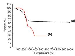
Fig. 1 TGA of (a)  $Re(\mu-S^iPr)_3(S^iPr)_6$  (1) and (b)  $[Mo(S_2CNEt_2)_4]$  (2) complexes.
