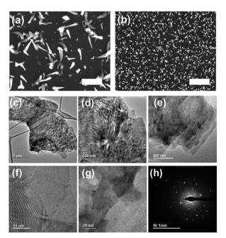
Fig. 4 Electron microscopy of rhenium disulfide (ReS<sub>2</sub>) thin films. (a) and (b) Secondary electron SEM images (10 kV) of thin films deposited by AA-CVD at 475 °C. Scale bars represent: (a) 2 μm; (b) 5 μm. (c-g) Bright field TEM images of ReS<sub>2</sub> thin films (200 kV). (h) Selected area electron diffraction pattern of an ReS<sub>2</sub> flake.
