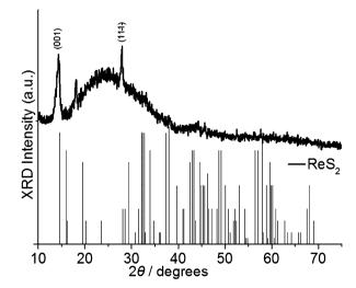
Fig. 2 Powder X-ray diffraction pattern for rhenium disulfide (ReS $_2$ ) deposited by AA-CVD using precursor (1) at 475 °C. The black sticks refer to the powder pattern of ReS $_2$  as reported by Wildervanck *et al.* <sup>46</sup> A simulated powder pattern is also available in the ESI.† The amorphous background is from the glass substrate.
