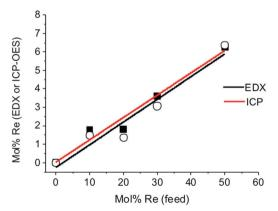
Fig. 5 Plot of mol% Re found in elemental analysis of  $Mo_{1-x}Re_xS_2$  (0  $\leq$  $x \le 0.06$ ) thin films produced by AA-CVD at 475 °C by EDX ( $\blacksquare$ ) and ICP-OE (O) spectroscopies as a function of varying mol% of Re in the AA-CVD
