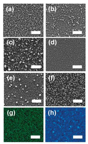
Fig. 8 Secondary electron SEM images (10 kV) of  $Mo_{1-x}Re_xS_2$  (0  $\leq x \leq 0.06$ ) thin films deposited at 475 °C by AA-CVD. (a) 0 mol% Re, (b) 1.79 mol% Re, (c) 1.80 mol% Re, (d) 3.60 mol% Re, (e) 6.25 mol% Re, and (f) ReS<sub>2</sub>; thin films were synthesized by using AA-CVD at 475 °C. EDX spectrum maps (30 kV) of (g) Mo  $L_{\alpha}$  and (h) Re  $K_{\alpha}$  emission in 1.8 mol% Re-doped MoS<sub>2</sub> films. All scale bars represent 5 µm.
