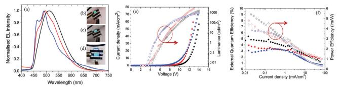
Fig. 11 (a) Normalized electroluminescent emission spectra of 1 (black), 2 (red) and 3 (blue) in thin films. Photograph of the working OLED with (b) 1 (c) 2 and (d) 3. (e) Current density and luminance *versus* applied voltage for OLEDs. (f) External quantum efficiency (solid circles) and power efficiency (open circles) *versus* applied voltage for OLEDs made with 1 (black) and 2 (red) and 3 (blue).
