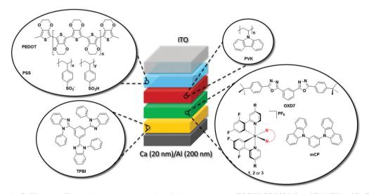
Fig. 10 Schematic for OLED device. The architecture consisted of the following structure: ITO/PEDOT: PSS (40 nm)/PVK (35 nm)/(mCP + active laver + OXD7) (30 nm)/TPBI (60 nm)/Ca (20 nm)/Al (200 nm) structure, where 1, 2 or 3 act as the active layer.
