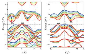
Fig. 2 Computed band structures of monolayer PtSe<sub>2</sub> under (a) isotropic compressive, and (b) isotropic tensile strain. The bands with different colors denote the band structures under different strain, *i.e.*, blue ( $\varepsilon=0\%$ ), cyan ( $\varepsilon=\pm2\%$ ), green ( $\varepsilon=\pm4\%$ ), yellow ( $\varepsilon=\pm6\%$ ) and red ( $\varepsilon=\pm8\%$ ). The Fermi level is located at 0 eV.
