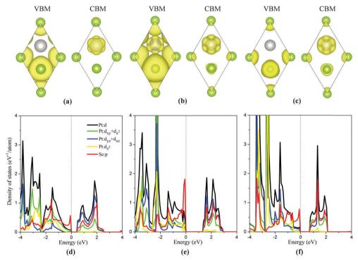
Fig. 3 Partial charge densities corresponding to the VBM and CBM, and partial densities of states (PDOS) of the monolayer PtSe<sub>2</sub> under isotropic strain of -8% (a and d), 0% (b and e) and 8% (c and f), respectively. Due to the specific symmetry, the contribution from  $d_{xy}$  is the same as that from  $d_{xz}$ , and the contribution from  $d_{yz}$  is the same as that from  $d_{xz}$ . The isosurface value is 0.001.
