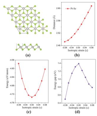
Fig. 1 (a) Top and side views of monolayer PtSe<sub>2</sub>. The green and gray balls represent Pt and Se atoms, respectively. (b) Pt-Se bond length versus isotropic in-plane strain. (c) Total energy per atom of the monolayer PtSe2 versus isotropic strain. (d) Computed band gap of monolayer PtSe2 versus isotropic strain.
