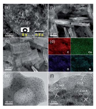
Fig. 1 (a and b) SEM images of the PCC sample. (c) SEM image, (d) the corresponding elemental mapping images, and (e and f) high-resolution TEM image of the PCC $-CoO_x$  sample. The inset in (a) illustrates fast wetting properties taken at 3 s after water droplet contact (0 s).
