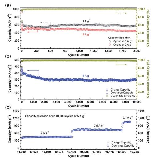
Fig. 5 Discharge/charge capacity and coulombic efficiency versus cycle number for the PCC-CoO<sub>x</sub> electrodes. (a) At current densities of 1 and  $2 \text{ A g}^{-1}$  for 2000 cycles. (b) At a current density of  $5 \text{ A g}^{-1}$  for 10 000 cycles after aging for five cycles at 0.1 A  $\text{g}^{-1}$ . (c) Subsequent capacity retention at various current densities from 2 to 0.1 A  $\text{g}^{-1}$  after 10 000 cycles at  $5 \text{ A g}^{-1}$ .
