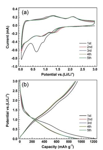
Fig. 3 (a) CV profiles of the initial five cycles at a scan rate of 0.2 mV s $^{-1}$  between 0.01 and 3.0 V. (b) Discharge/charge voltage profiles at a current density of 0.1 A g $^{-1}$  within a voltage window of 0.01–3.0 V for the first five cycles.
