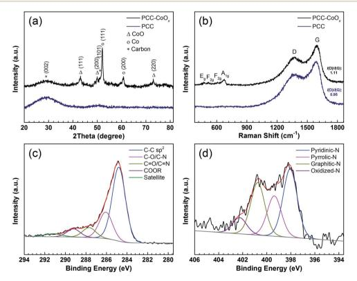
Fig. 2 (a) XRD patterns, and (b) Raman spectra of the PCC and the PCC-CoO<sub>x</sub> materials. High-resolution XPS spectra of (c) C 1s and (d) N 1s for the PCC-CoO<sub>x</sub> sample.
