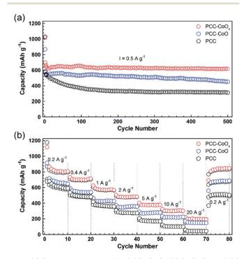
Fig. 4 (a) Cycling behaviours of the PCC–CoO $_x$ , PCC–CoO, and PCC electrodes at the same current density of 0.5 A g $^{-1}$ . (b) Rate performances of the PCC–CoO $_x$ , PCC–CoO, and PCC electrodes at various current densities ranging from 0.2 to 20 A g $^{-1}$ .
