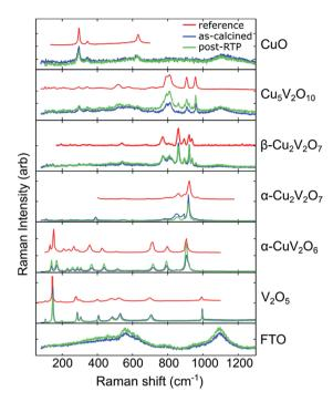
Fig. 2 Raman spectra identifying the presence of 6 phases in the composition libraries. Reference patterns of each phase are shown in red along with a representative Raman measurement from the ascalcined library (blue) and post-RTP library (green). An example pattern from the bare substrate is shown in the bottom panel.
