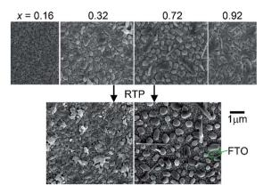
Fig. 1 SEM images of the representative as-calcined (top) and post-RTP (bottom) composition samples. Each sample is discontinuous and a bare FTO region is noted.
