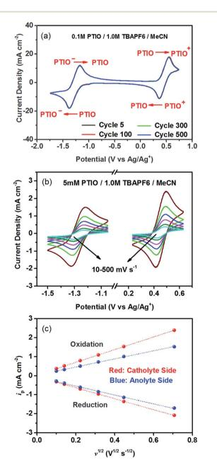
Fig. 1 CV curves of PTIO in a supporting electrolyte of 1.0 M TBAPF $_6$ / MeCN: (a) 500 cycles of repeated CV scans with 0.1 M PTIO at 100 mV s $^{-1}$ ; (b) at different potential sweep rates ( $\nu=10$ , 20, 50, 100, 200 and 500 mV s $^{-1}$ ) with 5.0 mM PTIO; (c) linear relationship between  $i_p$  and  $\nu^{1/2}$  obtained from Randles–Sevcik analysis.
