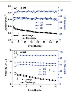
Fig. 3 Cycling efficiencies and capacities of the PTIO flow cells using a supporting electrolyte of 1.0 M TBAPF<sub>6</sub>/MeCN at a current density of 20 mA cm<sup>-2</sup>: (a) 0.1 M PTIO; and (b) 0.5 M PTIO.
