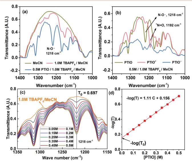
Fig. 4 FTIR of the PTIO species in the TBAPF<sub>6</sub>/MeCN electrolyte systems: (a) expanded spectral view for MeCN, 1.0 M TBAPF<sub>6</sub>/MeCN, and 0.5 M PTIO in 1.0 M TBAPF<sub>6</sub>/MeCN; (b) expanded spectral view of 0.5 M PTIO, PTIO<sup>+</sup>, and PTIO<sup>-</sup>; (c) expanded spectral view of PTIO in 1.0 M TBAPF<sub>6</sub> with [PTIO] ranging from 0.05 M to 0.5 M; (d) derived linear  $-\log(T)$  vs. [PTIO] calibration curve based on the peak at 1218 cm<sup>-1</sup>.
