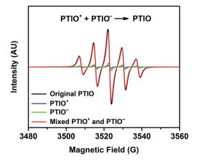
Fig. 2 ESR spectra of the original PTIO, PTIO $^+$ , PTIO $^-$ , and a mixture of PTIO $^+$  and PTIO $^-$  (1:1 volume ratio). PTIO $^+$  and PTIO $^-$  were electrochemically prepared by fully charging a flow cell employing the original PTIO electrolyte of 5.0 mM in 1.0 M TBAPF $_6$ . PTIO $^+$  and PTIO $^-$  do not have unpaired electrons and thus are not ESR active (the weak ESR signals in PTIO $^+$  and PTIO $^-$  belong to the small amount of unreacted PTIO).
