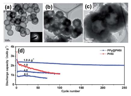
Fig. 11 TEM images of the (a) PHSi nanospheres, (b) PPy@PHSi nanocomposite and (c) PPy@PHSi electrode after 250 cycles at a current density of 1.0 A g<sup>-1</sup>. (d) Cycling performance of the PHSi and PPy@PHSi nanocomposite at a variety of current densities. Reproduced with permission.<sup>82</sup> Copyright 2014, John Wiley and Sons.
