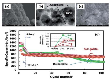
Fig. 10 (a) SEM and (b) TEM images of a Si/C-IWGN composite, and (c) SEM image of a particle cross-section of a Si/C-IWGN composite, and (d) cycling performances of Si/C and Si/C-IWGN composites (the inset shows electrode thickness increases of Si/C and Si/C-IWGNs electrodes during the 1st charge-discharge cycles). Reproduced with permission.74 Copyright 2015, Royal Society of Chemistry.
