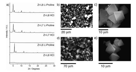
Fig. 2 (a) PXRD patterns showing the effects of incorporation of 5 equivalents of L-proline and one of HCl into solvothermal syntheses of Zr MOFs of L6-L8 compared to addition of HCl alone. SEM images of the MOFs formed using this protocol: (b) Zr-L5, (c) Zr-L6, (d) Zr-L7, (e) Zr-L8.
