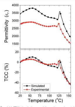
Fig. 6 Overlaid FEM simulation models and experimental data of temperature profiles for (a)  $\varepsilon_{\rm r}$  and (b) TCC. Excellent agreement is obtained showing the prediction of combining a BT core with 2.5% doped NNBT with  $V_{\rm f}=0.66$  provides potentially useful TCC behaviour.
