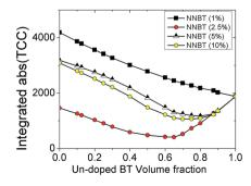
Fig. 5 The integrated absolute TCC response versus  $V_f$  of undoped BT for NNBT-BT ceramics based on Fig. 1. This provides a new method to identify the best combination of doped materials with undoped BT to minimise TCC in MLCCs.
