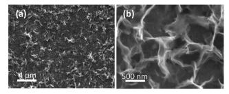
Fig. 6 SEM images of electrodeposited Co(OH)<sub>2</sub> on the Au electrode after the OER performed for 5 cycles under the conditions of Fig. 5.
