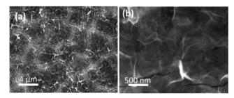
Fig. 2 (a and b) SEM images of Co(OH)<sub>2</sub> electrodeposited on to a Au electrode at a potential of -0.95 V for 60 s in a solution of 10 mM Co(NO<sub>3</sub>)<sub>2</sub>·6H<sub>2</sub>O.
