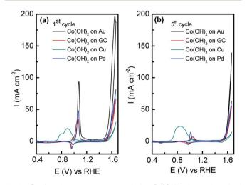
Fig. 5 Cyclic voltammograms recorded at  $Co(OH)_2$  electrodeposited on Au and GC electrodes and an unmodified Au electrode in 1 M NaOH recorded at 50 mV s<sup>-1</sup> showing (a) the first cycle and (b) the fifth cycle.
