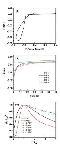
Fig. 1 (a) Cyclic voltammogram obtained at 50 mV s<sup>-1</sup> at a Au electrode in 10 mM Co(NO<sub>3</sub>)<sub>2</sub>·6H<sub>2</sub>O solution (b) current–time curves obtained at different applied potentials and (c) non-dimensional plots of  $(I/I_m)^2$  vs.  $t/t_m$  for the electrodeposition of Co(OH)<sub>2</sub>. Overlaid are the theoretical curves calculated using eqn (3) and (4) for progressive (—) and instantaneous (—) nucleation and diffusion limited growth.
