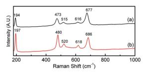
Fig. 4 Raman spectra of (a) as deposited Co(OH)<sub>2</sub> on Au and (b) after 5 cycles into the OER region.
