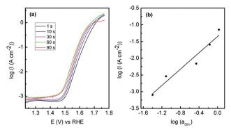
Fig. 7 (a) Tafel plots showing OER performance for Au/Co(OH)<sub>2</sub> electrodeposited from 10 mM Co(NO<sub>3</sub>)<sub>2</sub>·6H<sub>2</sub>O at different deposition time, (b) effect of hydroxide ion activity on OER. The cyclic voltammetric experiments used to obtain the data was recorded at a sweep rate of  $1 \text{ mV s}^{-1}$  in 1 M NaOH.
