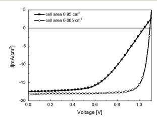
Fig. 6 J-V curves for the optimized  $CH_3NH_3Pbl_3$  perovskite layer with a small ( $A = 0.065 \text{ cm}^2$ ) and larger ( $A = 0.95 \text{ cm}^2$ ) electrode size. The solar cell in planar heterojunction architecture is composed by ITO/ PEDOT:PSS/PolyTPD/CH3NH3Pbl3/PCBM/3TPYMB/Au. Reproduced with permission from ref. 71.
