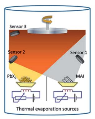
Fig. 4 Illustration of the dual-source vacuum deposition instrument. The PbX<sub>2</sub> (X = I, Cl) and  $CH_3NH_3I$  (MAI) precursors are thermally evaporated in vacuum. The deposition rate and thickness are monitored using quartz microbalances. Reproduced with permission from ref. 75.
