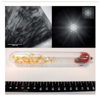
Fig. 2 Top left – Bright field transmission electron microscopy of an  $SnS_2$  platelet, image near the [0001] zone axis. Top right – Convergent beam electron diffraction pattern near the [0001] zone axis and, inset, detail of the zero order Laue zone from the same sample. Bottom centre – Macroscopic single crystals synthesised from the CVT method, with the scale in centimetres.
