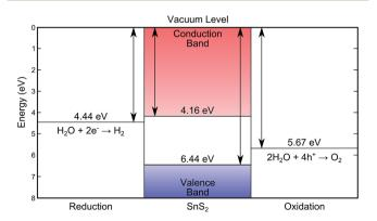
Fig. 4 The energy levels of SnS<sub>2</sub> as determined by XPS/IPES in this work, showing the desirable band placements for water splitting.7,8
