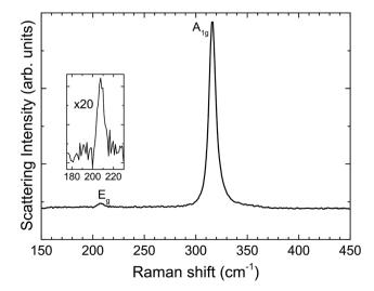
Fig. 3 Raman spectrum from  $\mathrm{SnS}_2$ , with  $\mathrm{A}_{1g}$  and  $\mathrm{E}_{g}$  modes indicative of the 2H polytype. The inset shows a 20 times magnification of the  $\mathrm{E}_{g}$  mode.
