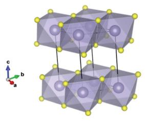
Fig. 1 Ground state (2H) structure of SnS<sub>2</sub> showing the 2-dimensional bonded plane of edge-sharing octahedra and the conventional unit
