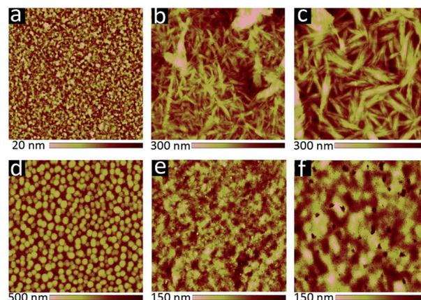
Fig. 4  $10 \times 10 \mu\text{m}$  AFM images of active layer blends cast from  $20 \text{ mg mL}^{-1}$  solutions; (a–c) **6**: $\text{PC}_{71}\text{BM}$  active layers with (a) 0%, (b) 1%, (c) 3% DIO (v/v); (d–f) **8**: $\text{PC}_{71}\text{BM}$  active layers with (d) 0%, (e) 1%, (f) 3% DIO (v/v).
