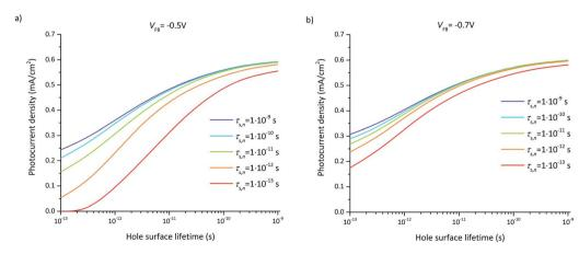
Fig. 11 Photocurrent density at 0.3 V vs. RHE as a function of the hole surface lifetime for various electron lifetimes ( $\tau_{s,n}=10^{-9}$ ,  $10^{-10}$ ,  $10^{-11}$ ,  $10^{-12}$ ,  $10^{-13}$  s) and two flatband potentials: (a)  $V_{FB}=-0.5$  V vs. RHE, and (b)  $V_{FB}=-0.7$  V vs. RHE.
