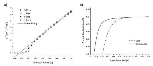
Fig. 5 (a) Mott-Schottky plot for four frequencies (500 Hz, 1 kHz, 5 kHz, 10 kHz) of a 1 μm thick nid-GaN sample immersed in 1 M H<sub>2</sub>SO<sub>4</sub> electrolyte under dark. (b) Experimental dark current density (dashed line) and photocurrent density (solid line) vs. RHE
