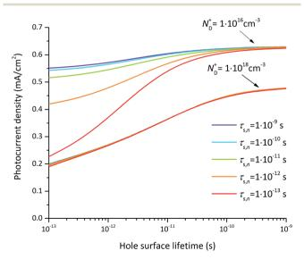
Fig. 9 Photocurrent density at 1.23 V vs. RHE as a function of the hole surface lifetime for various electron lifetimes ( $\tau_{s,n} = 10^{-9}$ ,  $10^{-10}$ ,  $10^{-11}$ ,  $10^{-12}$ ,  $10^{-13}$  s) and two doping concentrations ( $N_D^+ = 10^{16} \ \text{cm}^{-3}$  and  $N_{\rm D}^{+} = 10^{18} \, \rm cm^{-3}$ ).
