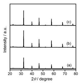
Fig. 1 XRD patterns for SrTiO<sub>3</sub> particles. (a) STO(pristine), (b) STO(flux-Y), and (c) STO(flux-Al).
