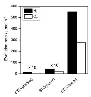
Fig. 3 Water splitting activity of  $SrTiO_3$  photocatalysts. Reaction conditions: catalyst, 0.1 g; cocatalyst,  $Rh_{2-y}Cr_yO_3$  (Rh 0.1 wt%, Cr 0.1 wt%); reaction solution, 100 mL  $H_2O$ ; light source, 300 W Xe lamp ( $\lambda > 300$  nm).
