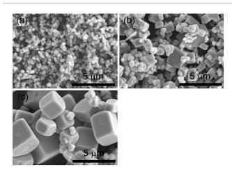
Fig. 2 SEM images of SrTiO<sub>3</sub> particles. (a) STO(pristine), (b) STO(flux-Y), and (c) STO(flux-Al).
