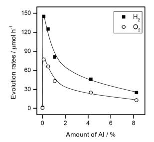
Fig. 6 Dependence of the water splitting activity of STO(ssr-Y) on the amount of Al doping. Reaction conditions: catalyst, 0.1 g; cocatalyst, Rh<sub>2-v</sub>Cr<sub>v</sub>O<sub>3</sub> (Rh 0.1 wt%, Cr 0.1 wt%); reaction solution, 100 mL H<sub>2</sub>O; light source, 300 W Xe lamp ( $\lambda > 300$  nm).
