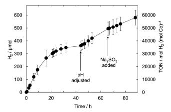
Fig. 3 Long-term photoactivity of the optimised QD-BF<sub>4</sub>/CoCl<sub>2</sub> system at 25 °C ([QD-BF<sub>4</sub>] = 2  $\mu$ M, [Co] = 4  $\mu$ M, 1.0 M Na<sub>2</sub>SO<sub>3</sub>, pH 7,  $\lambda$  > 420 nm, 100 mW cm<sup>-2</sup>).
