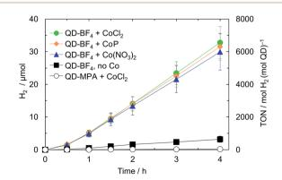
Fig. 2 Comparison of visible-light driven  $H_2$  evolution performance with mercaptopropionic acid-capped CdS (QD-MPA) and ligand-stripped CdS (QD-BF<sub>4</sub>) in the presence of various Co co-catalysts at 25 °C (0.1 M Na<sub>2</sub>SO<sub>3</sub>, pH 7, [QD-BF<sub>4</sub>] = 2  $\mu$ M, [Co] = 4  $\mu$ M, 2.5 mL, irradiation  $\lambda$  > 420 nm, 100 mW cm<sup>-2</sup>).
