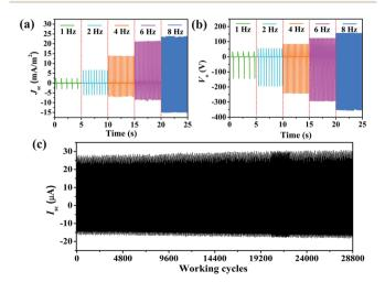
Fig. 4 (a)  $I_{\rm sc}$  and (b)  $V_{\rm o}$  of the PPy NW-based TENG in the frequency range from 1 Hz to 8 Hz. (c)  $I_{\rm sc}$  of the TENG working continuously for 28 800 cycles.
