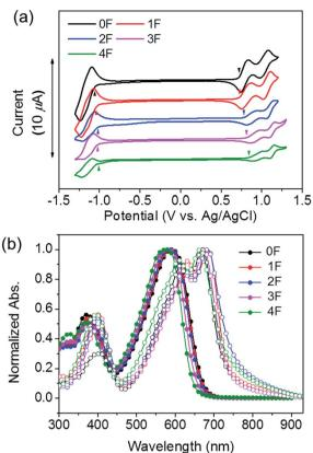
Fig. 1 (a) Cyclic voltammograms of 0-4F dichloromethane solutions containing 0.1 mol L $^{-1}$  Bu<sub>4</sub>NPF<sub>6</sub> and a scan rate of 50 mV s $^{-1}$ . (b) UV-vis absorption spectra of 0-4F chloroform solutions (filled circles) and films (open circles).
