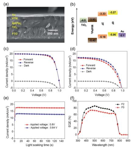
Fig. 7 (a) The SEM cross-section image and (b) energy diagram of the perovskite solar cell device. The current density-voltage (J-V) characteristics based on the solar cells with (c) **2F** and (d) **0F**. (e) current density (J) variation of the **0F** and **2F** based PSCs with a light soaking (1 Sun) time under the applied bias voltage  $(V_{opt})$  at maximum power point  $(P_{max})$  and (f) EQE spectra of the **0F** and **2F** based PSCs.
