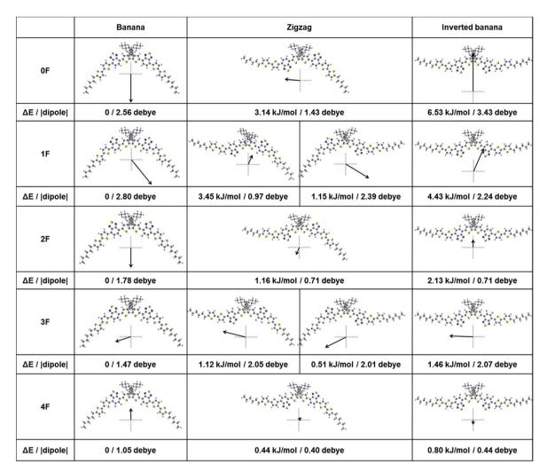
Fig. 6 Optimized molecular conformations, energy difference from the banana shape conformer of each compound and their dipole moments for compounds 0F-4F.
