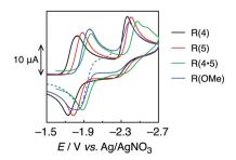
Fig. 2 Cyclic voltammograms of R(X) (0.5 mM) in DMF under Ar, measured with a 100 mV s<sup>-1</sup> sweep rate.
