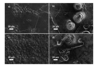
Fig. 6 Scanning electron microscopy images of a short-circuited Li anode after galvanostatic (a) polarization (0.40 mA cm<sup>-2</sup>) and (c) cycling (0.26 mA cm<sup>-2</sup>) test with hPNB-PEO electrolyte (plasticized with 32 wt% PEG 275) and (b) polarization (0.40 mA cm<sup>-2</sup>) and (d) cycling (0.26 mA cm<sup>-2</sup>) test with PCOD-PEO electrolyte (plasticized with 32 wt% PEG 275).
