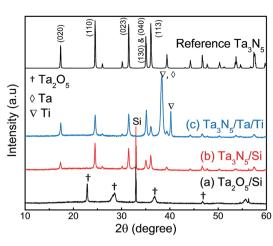
Fig. 2 XRD patterns for (a)  $Ta_2O_5/Si$  and (b)  $Ta_3N_5/Si$  obtained from the nitridation of  $Ta_2O_5/Si$ , and (c)  $Ta_3N_5/Ta/Ti$  after the transfer process. The standard pattern for the  $Ta_3N_5$  phase (PDF# 89-5200) is displayed at the top as a reference.
