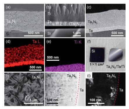
Fig. 3 Cross-sectional SEM images of (a)  $Ta_3N_5/Si$  and (b)  $Ti/Ta/Ta_3N_5/Si$ , (c) cross-sectional STEM image of transferred  $Ta_3N_5/Ta/Ti$ , EDS maps for (d) Ta and (e) Ti taken from the STEM image in panel (c), (f) digital photographs of a  $Ta_3N_5/Ta/Ti$  sample transferred from a Si substrate, (g) topview SEM image of a  $Ta_3N_5/Ta/Ti$  sample, and dark-field (h) STEM and (i) zone-axis TEM images of a  $Ta_3N_5/Ta/Ti$  sample near the  $Ta_3N_5/Ta/Ti$  interface.
