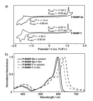
Fig. 3 (a) Cyclic voltammogram of P-BNBP-Se and P-BNBP-T in thin films using a Ag/AgCl reference electrode, Fc = ferrocene; (b) UV/Vis absorption spectra of P-BNBP-Se and P-BNBP-T in *o*-DCB solutions and in thin films.
