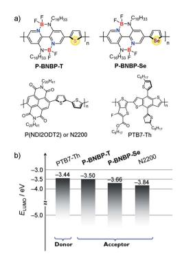
Fig. 1 (a) Chemical structures of P-BNBP-Se, P-BNBP-T, N2200 and PTB7-Th and (b) their LUMO energy level alignments.
