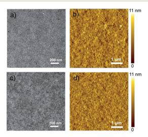
Fig. 6 The TEM images and the AFM height images of ((a) and (b)) the PTB7-Th:P-BNBP-Se blend and ((c) and (d)) the PTB7-Th:P-BNBP-T blend, respectively.
