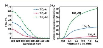
Fig. 5 (a) The incident photon-to-electron conversion efficiency (IPCE) values of TiO<sub>2</sub>-A (blue), TiO<sub>2</sub>-R (red) and TiO<sub>2</sub>-AR (green). (b) The carrier separation efficiencies of TiO<sub>2</sub>-A (blue), TiO<sub>2</sub>-R (red) and TiO2-AR (green).
