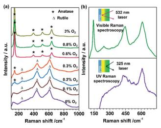
Fig. 2 (a) Visible Raman spectra of the  $TiO_2$  films fabricated at different  $O_2$  partial pressures. (b) Visible and UV Raman spectra of the  $TiO_2$ -AR electrode, which consists of an internal anatase phase  $TiO_2$  layer and external rutile phase  $TiO_2$  layer.
