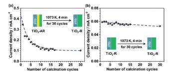
Fig. 6 Dependence of the current density values of TiO<sub>2</sub>-AR electrode (a) and TiO2-R electrode (b) on the number of calcination cycles. After calcination treatment at 1073 K for 120 min (4 minutes per cycle and 30 cycles), the TiO<sub>2</sub>-AR was converted to pure rutile phase.
