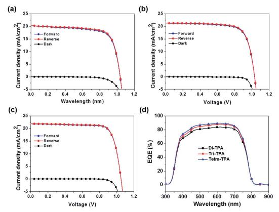
Photovoltaic properties of planar MAPbl<sub>3</sub> hybrid solar cells with (a) di-TPA, (b) tri-TPA, and (c) tetra-TPA and (d) EQE spectra.
