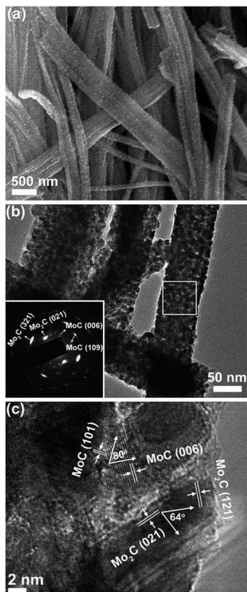
Fig. 2 (a) SEM, (b) TEM and (c) HR-TEM images of MoC–Mo<sub>2</sub>C-31.4 HNWs. Inset of (b) is the SAED pattern obtained on the marked area.
