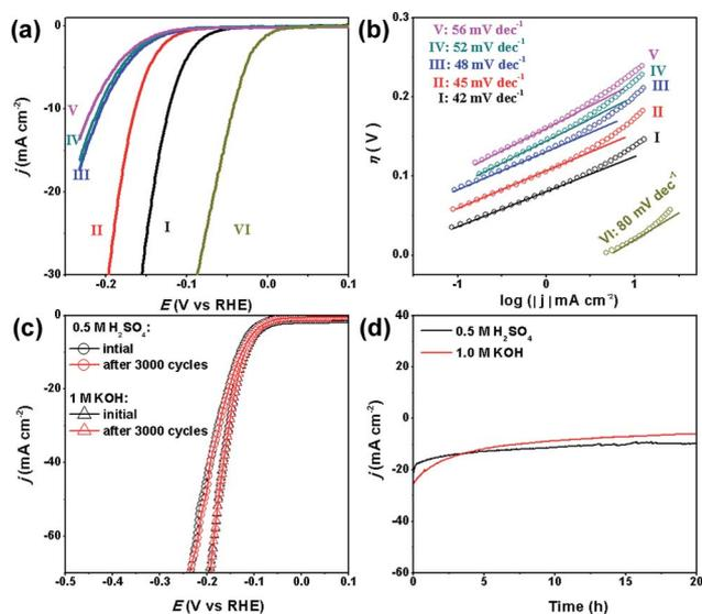
Fig. 5 (a) Polarization curves and (b) Tafel plots for the HER on modified GCEs comprising (I) MoC–Mo<sub>2</sub>C-31.4, (II) Mo<sub>2</sub>C, (III) MoC–Mo<sub>2</sub>C-68.1, (IV) MoC–Mo<sub>2</sub>C-30 (mixed), (V) MoC, and (VI) commercial Pt/C in 1.0 M KOH. (c) Stability of the MoC/Mo<sub>2</sub>C-31.4 modified electrodes with an initial polarization curve and after 3000 cycles in 0.5 M H<sub>2</sub>SO<sub>4</sub> and 1.0 M KOH, and (d) the long-term durability tests at  $\eta = 190$  mV.
