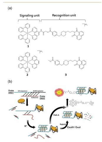
Fig. 1 (a) Chemical structure of Ir(III) complexes 1 and 2 and the G-quadruplex loop binder 3. (b) Schematic diagram illustrating the AGR2 sensing platform utilizing the DNA binder linked Ir(III) complex 1.
