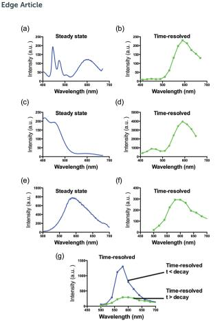
Fig. 2 Steady-state photoluminescence and time-resolved emission spectra of 1 in the presence of (a and b) perylene, (c and d) coumarin and (e–g) rhodamine B fluorescent media.
