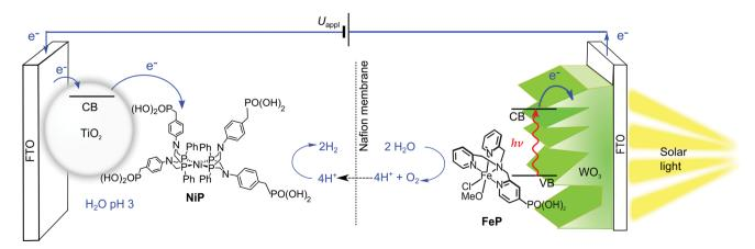
Scheme 1 Schematic representation of PEC water splitting with the  $TiO_2|NiP|$  hydrogen evolution cathode wired to the  $WO_3|FeP|$  oxygen evolution photoanode in an aqueous electrolyte solution at pH 3.
