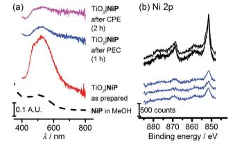
Fig. 6 (a) Diffuse-reflectance UV-vis absorption spectra of NiP-modified TiO $_2$  electrodes as prepared (red line), after 1 h PEC electrolysis at  $U_{\rm appl}=1.1$  V, and after 2 h CPE at  $E_{\rm appl}=-0.33$  V vs. RHE, with a MeOH solution UV-vis spectrum as a reference (dashed line). (b) X-ray photoelectron spectra in the Ni 2p region of TiO $_2$ |NiP and electrodes before (black line) and after (blue line) 1 h PEC electrolysis at  $U_{\rm appl}=1.1$  V with WO $_3$ |FeP.
