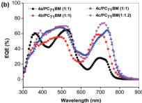
Fig. 2 The best J-V curves (a) and EQEs (b) of devices based on  $4a-c/PC_{71}BM$ .
