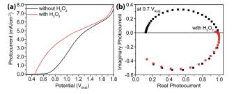
Fig. 6 Characterizations with H<sub>2</sub>O<sub>2</sub> as hole scavengers. (a) Steadystate current-voltage curves for sdH with (red) and without (black) H<sub>2</sub>O<sub>2</sub>. (b) IMPS data of sdH with (red) and without (black) H<sub>2</sub>O<sub>2</sub> at 0.7 V vs. RHE.
