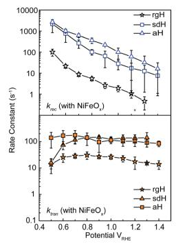
Fig. 3 Rate constants for hematite photoelectrodes with NiFeO $_{\rm x}$  surface decorations. Top: recombination rate constants for photoelectrodes by three different preparation methods; bottom: surface charge transfer rate constants for the same photoelectrodes. The error bars are standard deviations between different samples.
