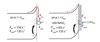
Fig. 8 Surface decorations on hematite improves the overall PEC performance by reducing surface recombination. Compared with bare hematite (left), NiFeO<sub>x</sub> does not change  $k_{tran}$  (right). Instead, it reduces the recombination rate constant  $(k_{rec})$  greatly.
