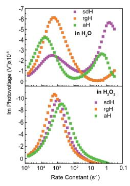
Fig. 7 Intensity modulate photovoltage spectroscopy (IMVS) of various hematite photoelectrodes in H<sub>2</sub>O (top) and in H<sub>2</sub>O<sub>2</sub> (bottom). Data presented as Bode plots, where the Y axis shows the imaginary component of the complex photovoltage, and the X axis shows the rate constants converted from the modulation frequencies
