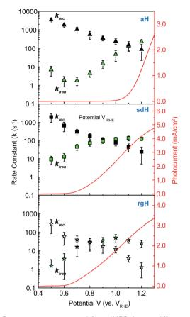
Fig. 2 Rate constants extracted from IMPS data at different applied potentials. Top: aH; middle: sdH; and bottom: rgH. Rate constants of recombination are shown as black symbols; rate constants for surface charge transfer are shown as green symbols. The error bar is the standard deviation between different samples (typically 4 to 5 samples are measured for each group of data).
