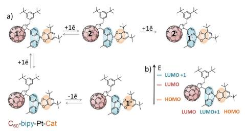
Scheme 3 (a) Schematic representation of the sequential electrochemical processes occurring in complex 3 upon reduction/oxidation and (b) corresponding qualitative energy level diagram for the frontier molecular orbitals deduced from cyclic voltammetry, spectroelectrochemical and EPR measurements (the HOMO, LUMO and LUMO+1 are located predominantly on the catecholate, fullerene and bipyridine moieties of the complex 3 respectively).
