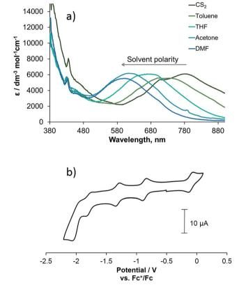
Fig. 1 (a) UV/vis absorption spectra of complex 3 recorded in solvents of different polarity and (b) the cyclic voltammogram of 3 in DMF with  $[^nBu_4N][BF_4]$  (0.2 M) as supporting electrolyte at a scan rate of 0.1 V s<sup>-1</sup>.
