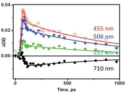
Fig. 6 Transient absorption spectra of 3 in THF solution observed upon laser excitation (355 nm) at room temperature. Left: the decay associated spectra obtained by global fit to the data using a cascade model  $A \to B \to C$ , (C = ground state);  $\tau_1 15 \, (\pm 6)$  ps,  $\tau_2 \, 890 \, (\pm 80)$  ps (see text for detail). Right: kinetic traces at selected wavelength (symbols) with the solid lines representing the two-exponential fit to the data using the parameters above.
