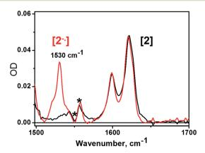
Fig. 3 IR spectra of 2 (black line) and electrochemically generated  $2^{1-}$  (red line) recorded in CH<sub>2</sub>Cl<sub>2</sub> solutions containing 0.2 M [ $^n$ Bu<sub>4</sub>N][BF<sub>4</sub>] electrolyte. The asterisks refer to incomplete solvent subtraction.
