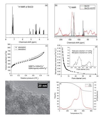
Fig. 1 (a) <sup>1</sup>H NMR spectrum of BnCD, (b) <sup>13</sup>C NMR of BnCD and solidstate <sup>13</sup>C NMR of BnCD-HCPP (spinning at 7 K), (c) N<sub>2</sub> adsorptiondesorption isotherms of BnCD-HCPP measured at 77 K (the polymer was pretreated at 170 °C under nitrogen flow for 2 h), (d) pore size distribution of BnCD-HCPP, (e) transmission electron microscope image of BnCD-HCPP, and (f) thermogravimetry and differential thermogravimetry curves of BnCD-HCPP.
