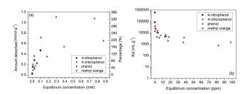
Fig. 2 Adsorption isotherms (a) and distribution coefficient (b) of BnCD-HCPP toward p-nitrophenol, p-chlorophenol, phenol, and methyl orange. The percentage in (a) was calculated as a molar percentage (mol/mol%) of the absorption amount (mmol g<sup>-1</sup>) to the amount of CD units (mmol  $q^{-1}$ ) in the adsorbent.
