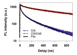
Fig. 3 Time-resolved PL decay kinetics for CuInS<sub>2</sub> core (blue dashed line) and CuInS2/CdS core/shell QDs (red dashed line) measured with 400 nm excitation. Their multi-exponential fits are shown in black solid lines and fitting parameters are listed in Table S1.†
