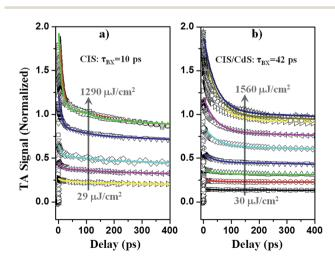
Fig. 5 Normalized exciton bleach TA kinetics (open symbols) at different excitation intensities for (a) CuInS<sub>2</sub> core, and (b) CuInS<sub>2</sub>/CdS core/shell QDs. The solid lines are fits to a multicarrier annihilation model described in the main text.
