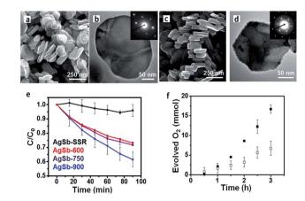
Fig. 7 (a) SEM and (b) TEM images of the NaSbO<sub>3</sub> product obtained from an aerosol-assisted synthesis. (c) SEM and (d) TEM images of the AgSbO<sub>3</sub>, single-crystalline NaSbO<sub>3</sub> plates in molten AgNO<sub>3</sub> were used as the template. (e) Rhodamine B photocatalytic degradation under  $\lambda = 400-500$  nm illumination. (f) Oxygen evolution in the presence of 0.1 M AgNO<sub>3</sub> (ref. 55 Copyright 2015, American Chemical Society).
