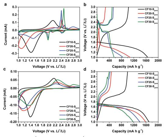
Fig. 5 The first CV scans at 0.1 mV s $^{-1}$  and GCD curves at 160 mA g $^{-1}$  of CF10-S $_{pore}$ , CF20-S $_{pore}$ , CF25-S $_{pore}$ , and CF30-S $_{pore}$  in TEGDME electrolyte (a) and (b) respectively, and in EC/DEC electrolyte (c) and (d), respectively.
