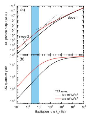
Fig. 2 Solutions of the TTA rate equations for typical rate constants of presently employed single-emitter TTA systems (black curve), and for a 10-fold increased TTA rate (red curve). The blue area highlights the range of sensitizer excitation rate achievable under sunlight illumination. It can be seen that upon increasing the TTA rate, the UC quantum yield under 1 sun conditions is significantly enhanced.
