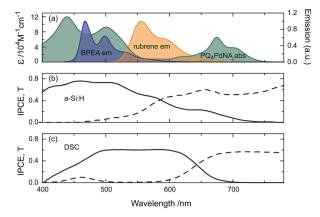
Fig. 3 The spectral properties of the two UC/device assembles in this study: (a) absorption of  $PQ_4PdNA$  (green) and emission of rubrene (orange) and BPEA (blue). IPCE (solid) and transmittance (dash) of (b) a-Si:H, illuminated through glass substrate and (c) DSC, illuminated through working-electrode.
