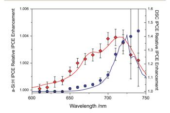
Fig. 5 Relative enhancement trace for a-Si:H device ( $\diamondsuit$ , red trace) tested with  $\sim$ 1.4 suns equivalent illumination ( $\lambda=670\pm5$  nm) and a DSC ( $\circ$ , blue trace) tested with  $\sim$ 1.3  $\odot$  equivalent illumination, including the modeled traces for the two devices.<sup>40,41</sup>
