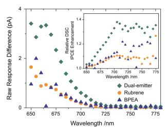
Fig. 4 Extra current generated from a DSC due to TTA-UC with dualemitter (green), rubrene only (orange) and BPEA only (blue) UC system. The inset shows the IPCE enhancement of the DSC with the three different UC systems.
