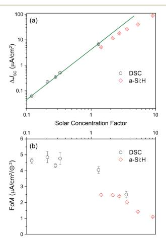
Fig. 6 (a) Dependence of calculated current gain ( $\Delta J_{SC}$ ) on effective solar concentration (both axes on a logarithmic scale) for the a-Si:H device (♦) and DSC (•). (b) Figure of merit (FoM) as a function of solar concentration for a-Si:H (♦) and DSC (•).
