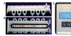
Fig. 1 The optoelectronic nose. (A) The linear array of colorimetric sensors and disposable cartridge. Cartridge side view (7.9  $\times$  2.8  $\times$  1.0 cm). (B) Cartridge front view. (C) Handheld reader/analyzer (12.8 imes 9.5 × 4.0 cm) based on a color contact line imager.
