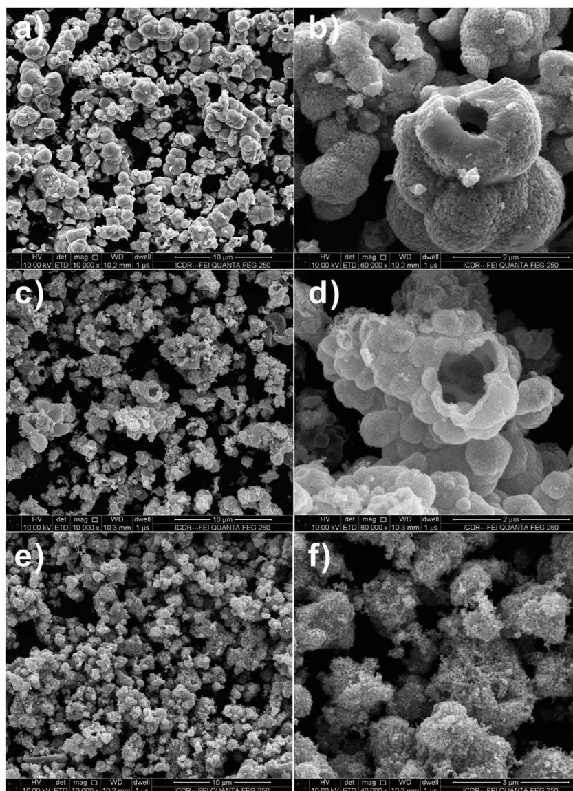
Fig. 2 FESEM images of SnO<sub>2</sub> samples after calcination at 550 °C for 3 h with 1 : 2 molar ratio of D-glucose and metal salt. (a and b) Na<sub>2</sub>SnO<sub>3</sub>·3H<sub>2</sub>O, (c and d) SnCl<sub>2</sub>·2H<sub>2</sub>O and (e and f) SnCl<sub>4</sub>·5H<sub>2</sub>O.
