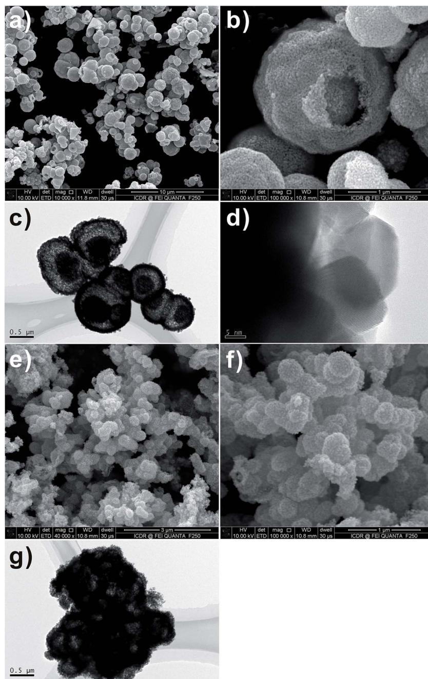
Fig. 5 FESEM and TEM images of  $\text{SnO}_2$  samples after calcination at  $600^\circ\text{C}$  for 3 h with 1 : 1 molar ratio of sucrose and metal salt. (a–d)  $\text{SnCl}_4 \cdot 5\text{H}_2\text{O}$  and (e–g)  $\text{SnCl}_2 \cdot 2\text{H}_2\text{O}$ .
