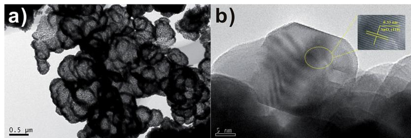
Fig. 4 (a) TEM (b) HRTEM images of  $\text{SnO}_2$  samples after calcination at  $550^\circ\text{C}$  for 3 h with 1 : 2 molar ratio of  $\text{D-glucose}$  and  $\text{SnCl}_2 \cdot 2\text{H}_2\text{O}$ .
