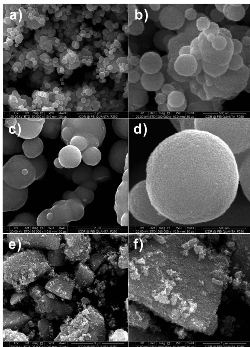
Fig. 3 FESEM images of  $\text{SnO}_2$  samples after calcination at 550 °C for 3 h with 1 : 0.4 molar ratio of D-glucose and metal salt. (a and b)  $\text{Na}_2\text{-SnO}_3 \cdot 3\text{H}_2\text{O}$ , (c and d)  $\text{SnCl}_2 \cdot 2\text{H}_2\text{O}$  and (e and f)  $\text{SnCl}_4 \cdot 5\text{H}_2\text{O}$ .
