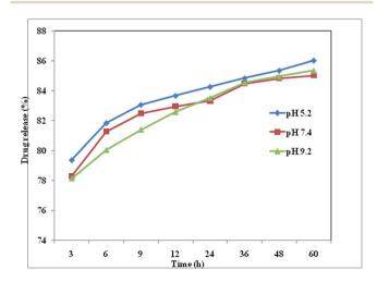
Fig. 4 Boldine drug release (%) from boldine-loaded CDs in PBS with pH values of 5.2, 7.4 and 9.2 at 37  $^{\circ}$ C.
