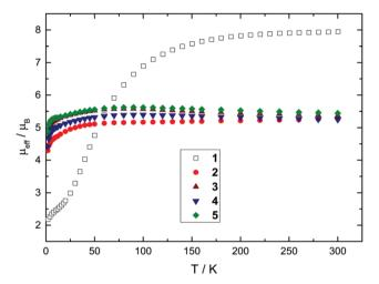
Fig. 2 Effective magnetic moment  $\mu_{\rm eff}$  vs. T plots for 1 and NHCadducts 2-5 (recorded in an applied magnetic field of 0.1 T).
