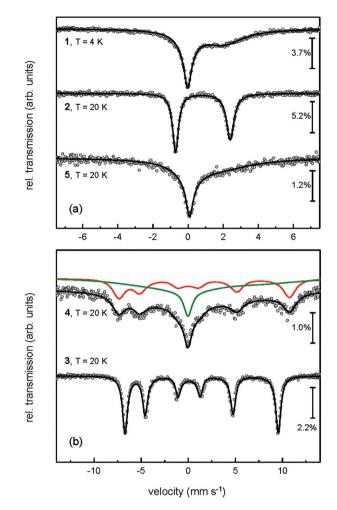
Fig. 5 Zero-field Mössbauer spectra of complex 1 measured at T = 4 K and NHC-adducts 2-5 recorded at T=20 K.
