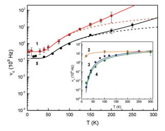
Fig. 6 Temperature-dependent relaxation rates  $\nu_c = \tau_c^{-1}$  for complexes 1-5. The broken lines consider only the spin-spin and Orbach relaxation term of ean (1) to illustrate the different contributions from Orbach and Raman type spin-lattice relaxation mechanisms. The full line represents the result of a least-squares fitting routine based on eqn (1).
