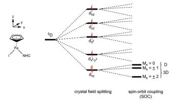
Fig. 4 Schematic illustration of the crystal field splitting and spin-orbit coupling for the <sup>5</sup>D (3d<sup>6</sup>) term.
