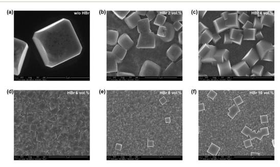
Fig. 2 SEM images of the top surfaces of the MAPbBr<sub>3</sub> layers deposited using 0-10 vol% of HBr in the DMF/HBr cosolvent on PEDOT:PSS-coated ITO/glass substrates.
