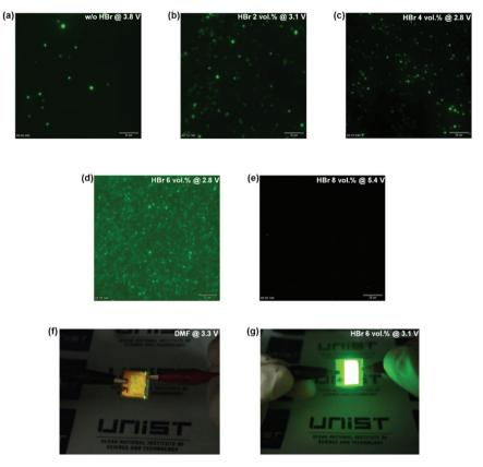
Fig. 3 (a-e) Optical microscopy images of EL from PeLEDs with the MAPbBr<sub>3</sub> layers deposited at a constant voltage using different concentrations of HBr in the DMF/HBr cosolvent. (f and g) 1 cm<sup>2</sup>-area green EL from MAPbBr<sub>3</sub> PeLEDs without and with 6 vol% of HBr in the DMF/HBr cosolvent, respectively.
