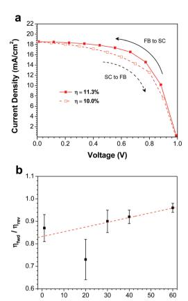
Fig. 5 (a) J-V curves measured at  $0.1 \, \mathrm{V \, s^{-1}}$  for the best device prepared at 40% RH. (b) Ratio of PCEs determined from forward (SC-FB) and reverse (SC-FB) scans as a function of RH. The linear fit is a guide to the eye.
