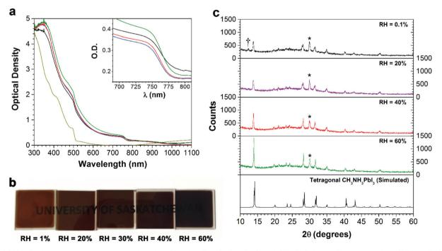
Fig. 2 (a) UV-Vis absorption spectra for vapor deposited  $Pbl_2$  thin films (yellow line), and  $CH_3NH_3Pbl_3$  thin films prepared at 1% (black line), 33% (blue line), 40% (red line), and 60% (green line) RH. (b) Photographs of  $CH_3NH_3Pbl_3$  thin films prepared at various RH values. (c) Powder X-ray diffraction patterns for  $ITO/Pbl_2/CH_3NH_3Pbl_3$  thin films prepared at various RH values. Peaks due to ITO and  $Pbl_2$  are marked with an asterisk (\*) and dagger (†), respectively.
