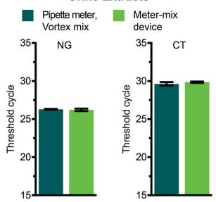
Fig. 4 qPCR threshold cycles on DNA extracted from urine spiked with either inactivated *Chlamydia trachomatis* (CT) or *Neisseria gonorrhoeae* (NG). Sample metering and mixing with lysis buffer was performed with either the meter-mix device (light green bars) or standard pipette and vortex (dark green bars). The remainder of the extraction protocol was identical for both conditions.
